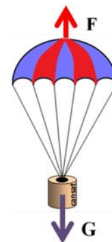
Figure 7. The structure of the CanSat parachute.
